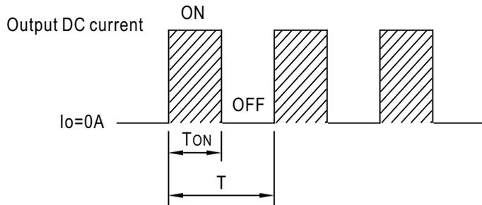
$$\text{Duty cycle(\%)} = \frac{T_{ON}}{T} \times 100\%$$
