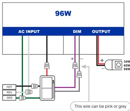
**Wiring from power supply to light fixture must be two conductor cable**
